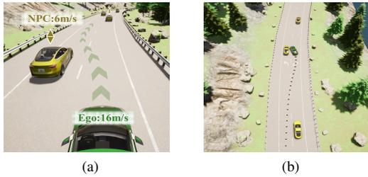
Fig. 1. (a) The traffic scenario created for the lane changing and overtaking tasks in CARLA. Green arrows indicate the safe and legal driving waypoints generated by a path planner for the driving agent to follow. (b) The victim vehicle side collides with an NPC vehicle. The black dash line indicates the driving route lasting for 3 seconds.
