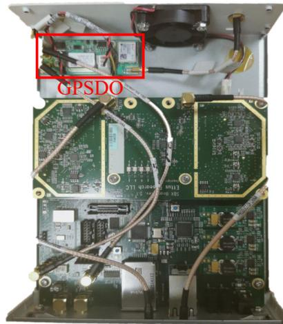
Fig. 20. USRP N210 with GPSDO. The GPSDO module is marked with a red rectangle.
