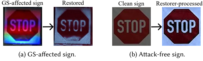
Fig. 23. The processing effect of the restorer on GhostStripe-affected and attack-free traffic signs.
