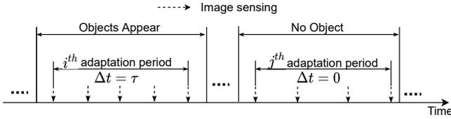
Fig. 9. Image sensing workflow for industrial product object tracking.
