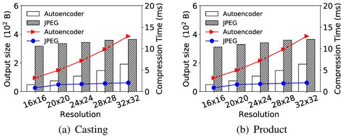
Fig. 6. Impacts of image resolution on output size and compression time under JPEG-10 and encoder with  $s_f = s_o = 3$ . The bars and lines represent output size and compression time, respectively.
