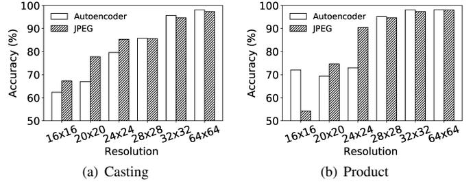
Fig. 5. Impacts of image resolution on image classification accuracy under JPEG-10 and encoder with  $s_f = s_o = 3$ .
