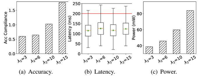
Fig. 15. Execution results under various settings of  $\lambda_2$  and  $\lambda_1 = 1$  and  $l_{th} = 200$ ms. The red line in (b) represents the  $l_{th}$ .
