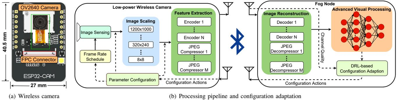
Fig. 2. EFCam system overview. A fog node can support multiple low-power wireless cameras at the network edge.
