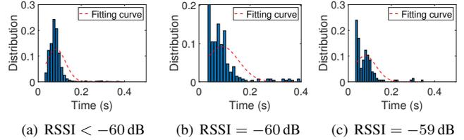
Fig. 12. Histograms and fitted Gaussian distributions for packet transmission latency under different RSSI levels. Results for the RSSI levels greater than  $-59$  dB are not shown.
