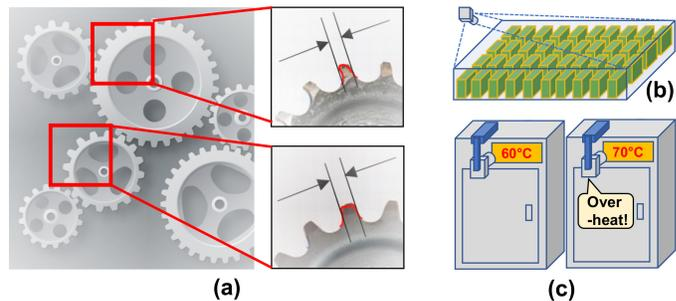
Fig. 1. Industrial vision applications. (a) Wear and tear assessment for gears; (b) Item counting; (c) Legacy equipment setting and condition monitoring. (The subfigure (a) is designed using resources from Freepik.com and Wikimedia Commons.)
