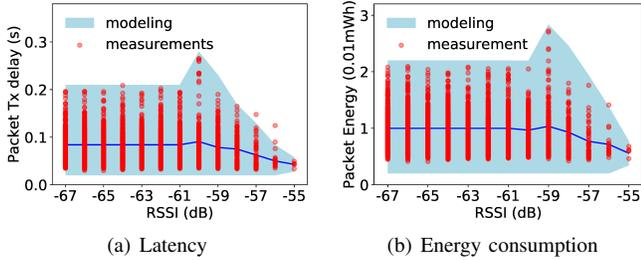
Fig. 11. Impacts of the RSSI on packet transmission latency and energy consumption. The line and belt represent the mean value and the  $\pm 3$  standard deviation of the fitted Gaussian distributions, respectively.
