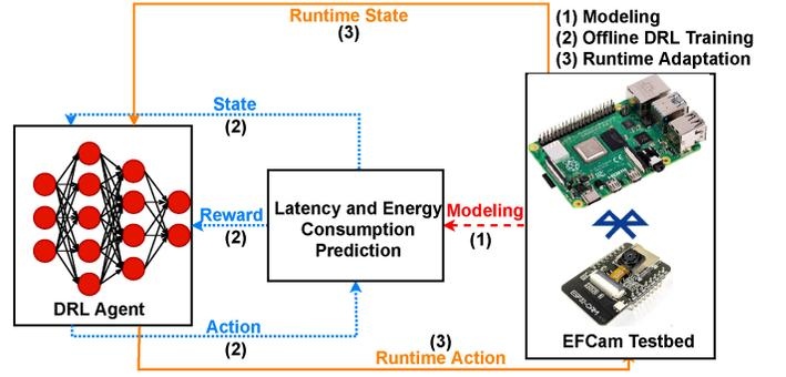
Fig. 10. Workflow of DRL-based adaptation.
