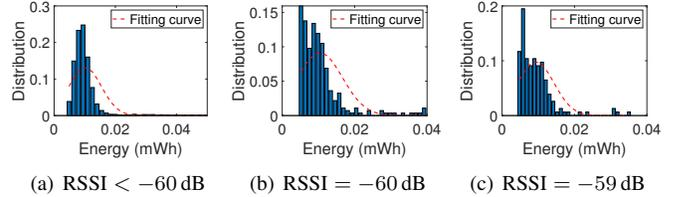
Fig. 13. Histograms and fitted Gaussian distributions for the camera energy consumption under different RSSI levels. Results for the RSSI levels greater than  $-59$  dB are not shown.
