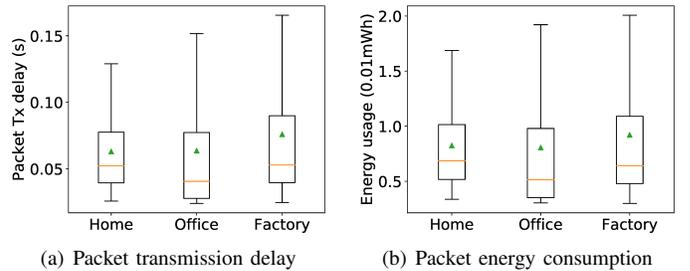
Fig. 8. Performance of BLE data transmission in different environment conditions. The box, line, triangle, upper and lower whiskers represent middle 50%, median, average, ranges for the bottom 25% and the top 25% of the samples, respectively.
