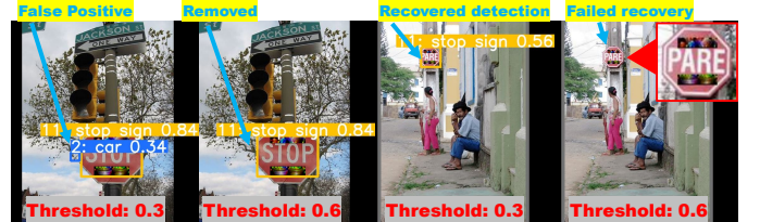
Fig. 2: Illustration of the trade-off between robustness and FPR under an adversarial attack on a stop sign. Raising the confidence threshold removes an undesired false positive (left) but hinders the recovery of the victim stop sign that would otherwise be detected at the lower threshold (right). Bounding boxes for other correct detections are omitted for readability.
